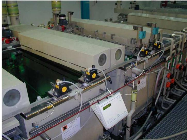
**Figure 4.4:** Two tanks for electroless nickel reaction. Behind there are two bars of PWDs immersed for deposition [14]
